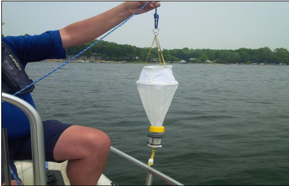
Figure 45. A zooplankton collection tow net (RLS).
